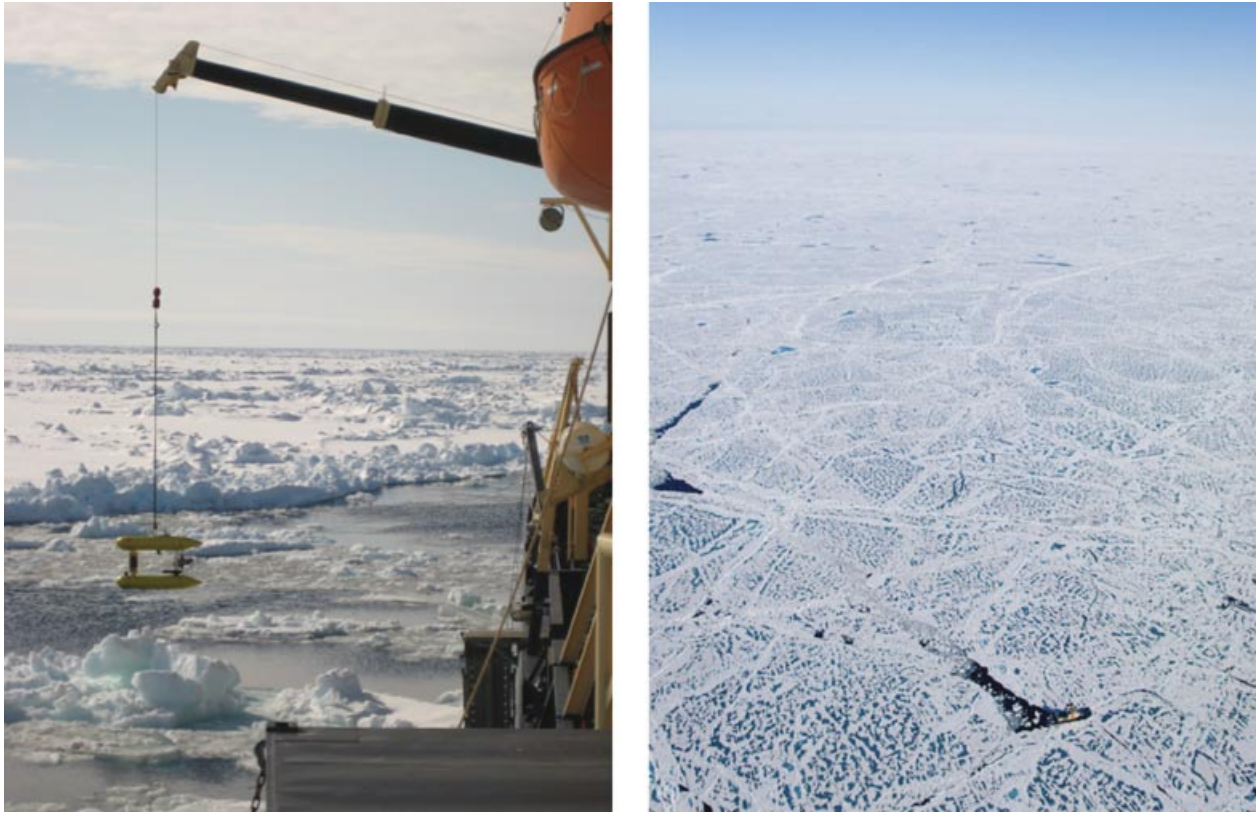
Figure 6. A typical deployment scenario for the AUV consisted of an open lead or pond into which the vehicle was released. The leads often contained large broken pieces of ice. The aerial view on the right shows a common case, in which the icebreaker (lower-right corner) copes with 90% or greater ice cover. The ship's trail of broken ice leads upward and to the left. The small dark shapes on the ice are surface melt ponds, not openings in the ice.
