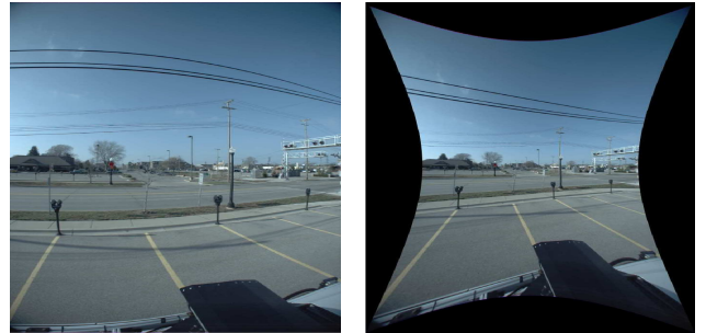
Fig. 6. The left panel shows a spherically distorted image obtained from the Ladybug3 camera. The right panel shows the corresponding undistorted image obtained after applying the transformation provided by the manufacturer.
