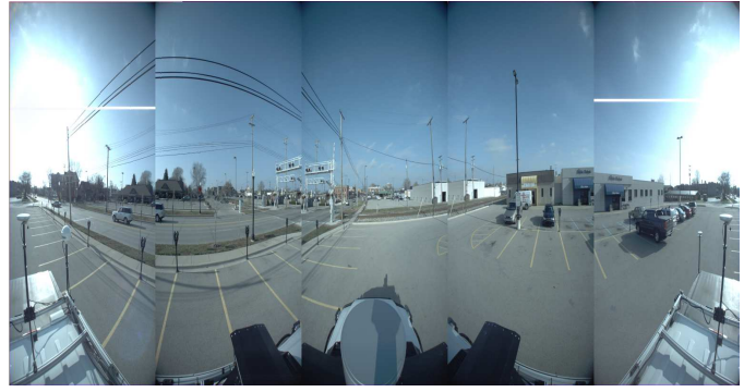
Fig. 5. The distorted images, from the five horizontal sensors of the omnidirectional camera, stacked together.
