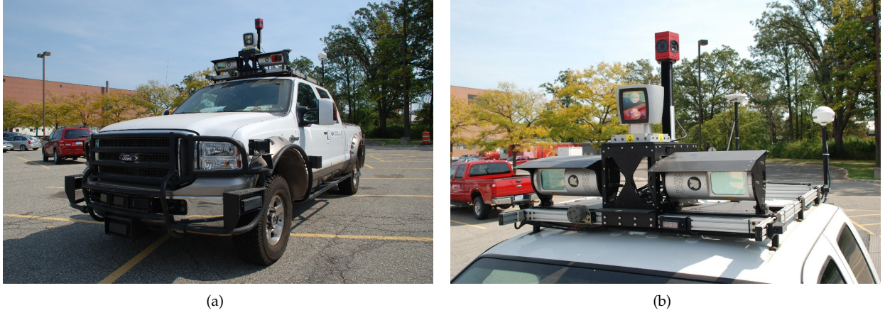
Figure 8: (a) The modified Ford F-250 pickup truck with sensor configuration as described in [Pandey et al., 2011b]. (b) The Velodyne HDL-64E 3D laser scanner [Velodyne, 2007] and the Point Grey Ladybug3 omnidirectional camera [Point Grey Research Inc., 2009] are mounted on the roof of the vehicle.
