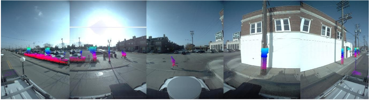
(b) Omnidirectional image with a subset of lidar points projected
