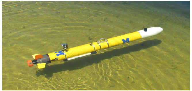
Fig. 4: Ocean Server, Inc., Iver2 AUV used during field trials at the University of Michigan Biological Station. Sensors include a 600 kHz Teledyne RDI Explorer DVL, a Microstrain 3DM-GX25 AHRS, and a Desert Star SSP-1 pressure-depth sensor
