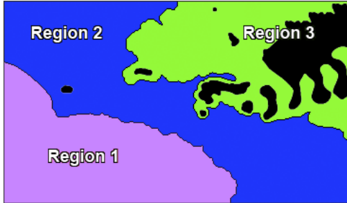
Fig. 6. Segmentation of the bathymetric map shown in Fig. 4 with n = 3 regions, with the workspace obstacles shown in black
