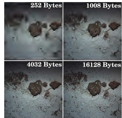
Fig. 6. The same image encoded at four different sizes using SPIHT. 81% of the transmitted data is used to reconstruct the luminance; the rest describes the image color channels.
