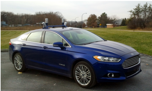
Fig. 4: Our autonomous car platform, a Ford Fusion equipped with four LIDAR units, survey-grade INS, and a steering interface able to operate in both SWA and steering torque mode. All perception and control is performed onboard.
