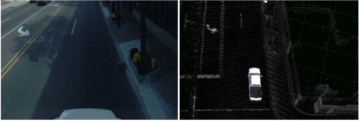
Figure 3.8 Counterexample showing that non-uniform lighting can play a critical role in influencing reflectivity/intensity correlation. (left) Ambient lit image with shadows of trees and buildings on the road. (right) Top view of the corresponding lidar reflectivity map, which is unaffected by ambient lighting due to its active lighting principle.
