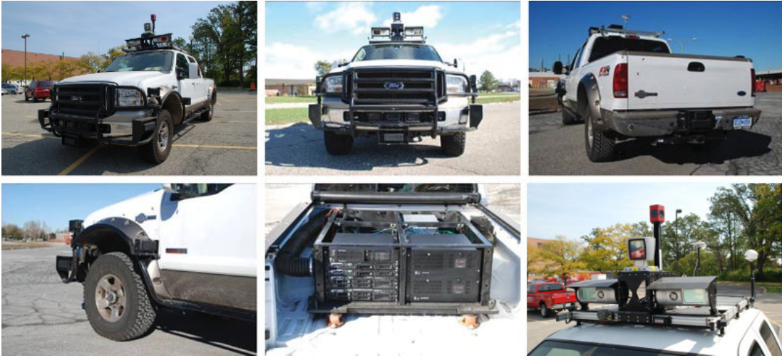
Figure 1.1 A collage of the modified Ford F-250 truck used in DARPA Grand Urban Challenge showing the sensor configuration and the computers. Sensors are strategically placed around the vehicle. The lidar and omnidirectional camera are mounted on top so that an entire 360 degree view of the environment is captured.
