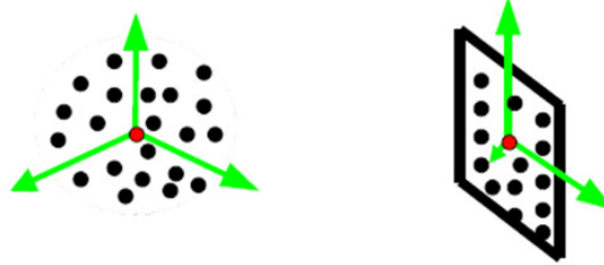
Figure 4.3 Local neighborhood structure of 3D points used in GICP algorithm [146] is captured by the sample covariance matrix. Planar surfaces show two dominant eigen-vectors of the sample covariance matrix (right). Uniformly distributed points show equal eigen-vectors in all three dimensions (left).
