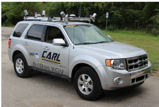
Fig. 6: Test platform used for experimental results. This platform is a TORC ByWire XGV equipped with 4 Velodyne HDL-32E LIDAR scanners and an Applanix POS-LV 420 INS.
